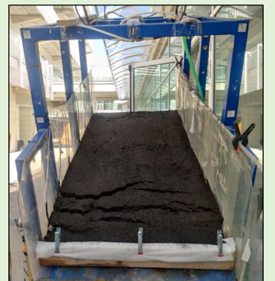
Cracks opening after rainfall test on burnt soil.
