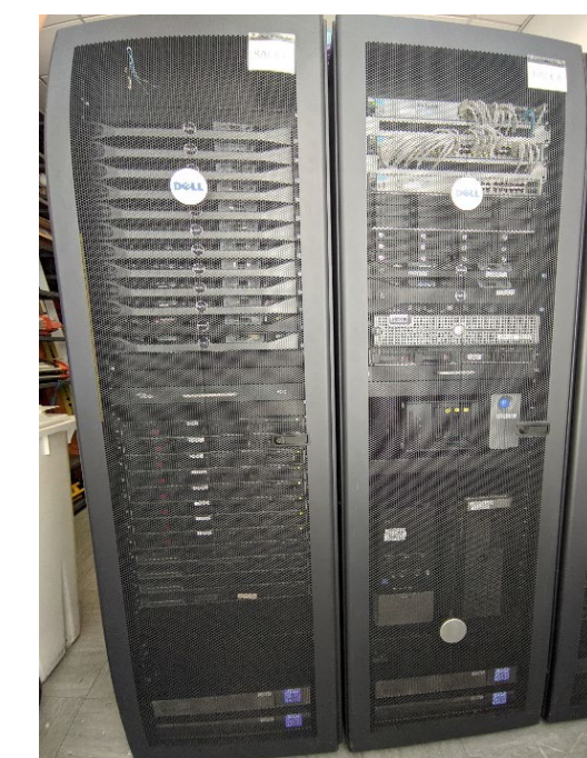
Fig. 6: Metashape processing cluster was composed of 9 parallel HP ProLiant SE1102 servers, with the following characteristics:
